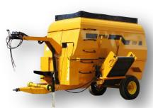
The mixer has a control lever located on the goose to activate the download and distribution of feed in the hopper , you must maneuver a lever to open the door , another to activate the band when you go to deposit the mix in the forage feeders and another to lower or raise the band.
